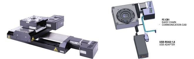
Once the controller address of each stage is set, unplug all the power cables and disconnect the USB cable from all the stages except for the FC controller that has its address set to 1. Use the daisy chain cables to connect each controller. For stages #2 thru 4, it does not matter whether you use the upper or lower RS422 connector to daisy chain.
